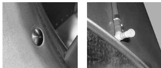
Measuring connector in inlet cone Hose pipe to connecting piece in the side wall Connecting piece (external diameter of 6mm) for the pressure measurement
